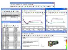
DynaTherma is coupled to DynaWorks RealTime which allows to manage the measurement points and monitor the thermal tests. Each test can be split in several phases for a better monitoring of the overall test campaign during several months. An advanced alarm tool allows to control the test results. For more information on DynaWorks RealTime, please consult us.
